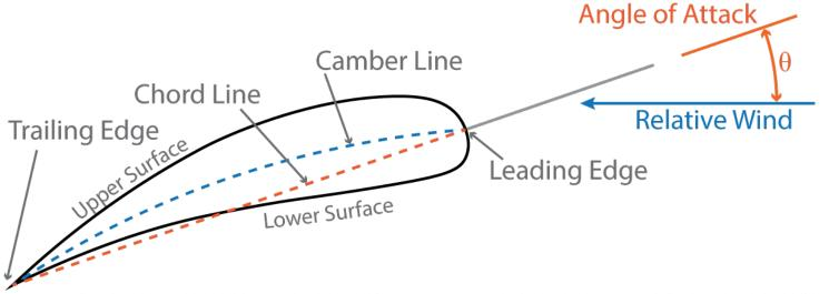
Leading Edge - the part of the airfoil that meets the relative wind first ٠ Trailing Edge - the part of the airfoil where the airflow of the upper surface and lower surface rejoin
